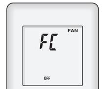
If no buttons are pressed within 30 seconds after the "FC" status is displayed, the system returns to the original clock display. In this case, start again from step 1.
