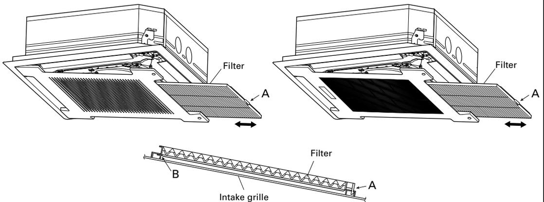
When reinstalling the filter, be sure that the hooks at A and B engage correctly into place.
