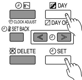
Press the DAY (DAY OFF) button and SET button simultaneously for 2 seconds or more to activate the part lock function and lock all of the buttons on the remote controller except the Start/Stop button, Set Temperature buttons, Master Control button, and Fan Control button. Press the buttons again for 2 seconds or more to deactivate the part lock function.
