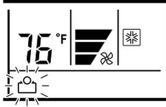
Press the ENERGY SAVE button to start or stop the energy-saving air conditioner operation.
