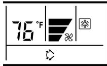
Press the vertical airflow direction and swing button.
