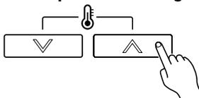
Press the SET TEMPERATURE buttons to set the temperature (from 64 °F to 88 °F).
