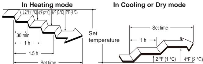
After the set time has elapsed, the air conditioner operation turns off.
