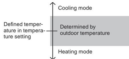
When Auto mode is first selected, the fan will operate at low speed for about a few minutes, during which time the indoor unit detects the room conditions and selects the operation mode.
