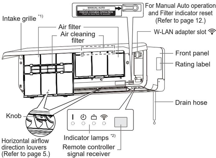
\*1) Before starting operation, make sure that the intake grille is closed completely. Incomplete closing may affect the proper function or performance of the product.
