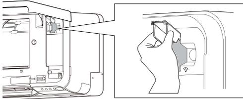
4. Plug the W-LAN adapter into the connection slot of the indoor unit in the direction as shown in the figure.
