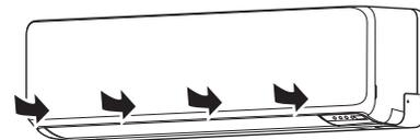
**NOTES:** If dirt accumulates on the air filter, airflow will be reduced, operating efficiency will lower, and the noise will increase.
