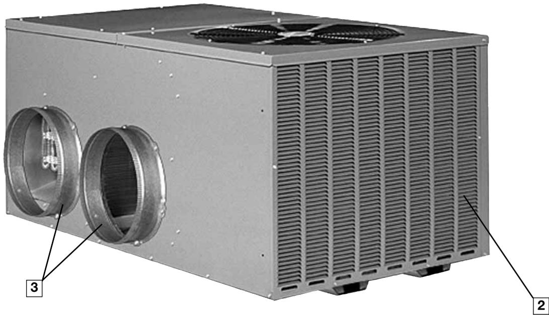
To provide flexibility in space-limited installations, the unit can be installed flush to the structure without blocking airflow over the outdoor coil or making any screws inaccessible for maintenance. Furthermore, the cabinet is a slim 33" wide. Full-louver coil protection (2) makes Fujitsu unique in the industry and also totally protects the outdoor coil from vandalism and weather extremes.
